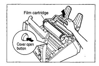
Remove the film stopper from the new film cartridge by pushing it up.
