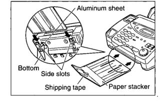
Confirm that the paper stacker is locked into the center slots and slide back.
