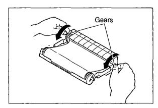
**5** Turn the film cartridge over so that the "BACK" is facing up.
