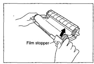
If the film is slack, tighten it by winding the gears.
